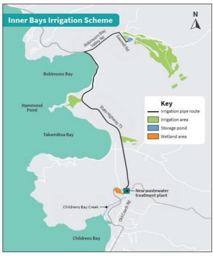
Figure 2-1: The Inner Bays Irrigation Scheme Concept
