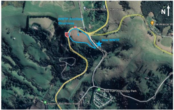
Figure 2: Hay Paddock Site on Old Coach Road, north of Akaroa, showing new WWTP location and associated ancillary structures including wetland, untreated water tank and pump shed.
