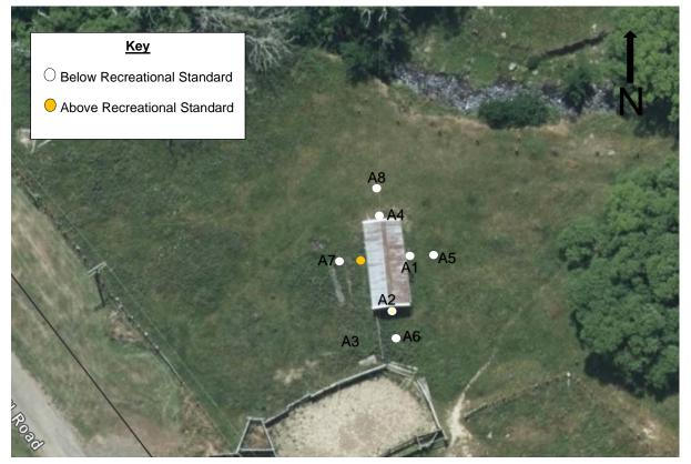
Figure 17: Farm Building A test locations. Samples FB A5- FB A8 were collected approximately 5m from the wall of the building. Note the stock pens to the south were assessed as being modern cattle pens and not a HAIL site.
