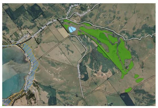
Figure 56. Indicative location of native planting irrigation areas (in green) and gravity pipeline (in yellow) from the CH2m Beca Report (2020: Appendix J). Note the plan shows storage ponds which are no longer proposed, with storage tanks proposed instead.
