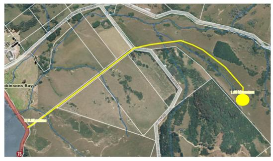
Figure 55. Indicative location of gravity fed pipeline and storage tanks on the hillside at 11 Sawmill Road (Client provided image).
