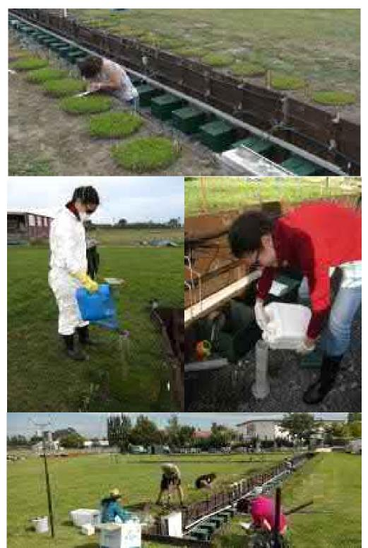
Fig. 3. Top: The installed lysimeters showing the six Pawson silt loam soil cores (front-left) and the 12 Barry's soil cores (rear-right). Centre left: Effluent application. Centre right: Drainage collection. Bottom: Destructive sampling of the lysimeters at the conclusion of the experiment. 16<sup>th</sup> of November, 2016.
