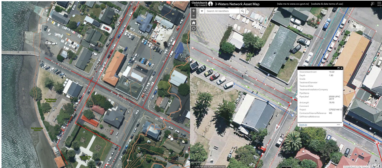
Figure 2: Images from Canterbury Maps GIS data – highlighting lower-lying areas of gravity WW network with invert levels of approximately RL1m.
